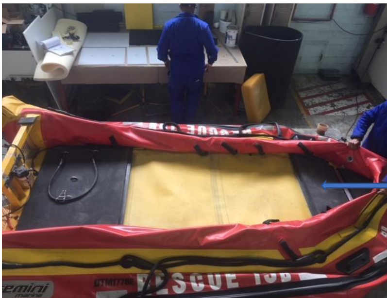
Bow boards fitted with stringer in between and under the floor board retaining rubber. Stringer is the right way up.
