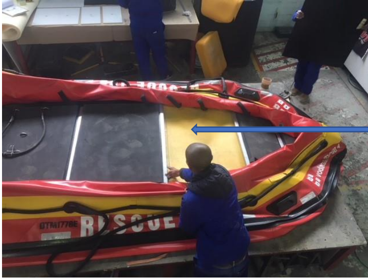
Stringers fitted to fourth and second floorboards.
