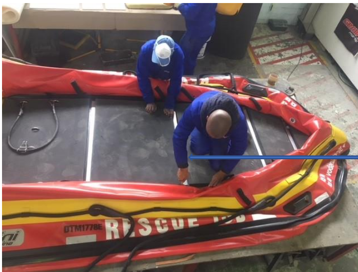
Floorboards being worked underneath retaining rubber using a metal bone.
