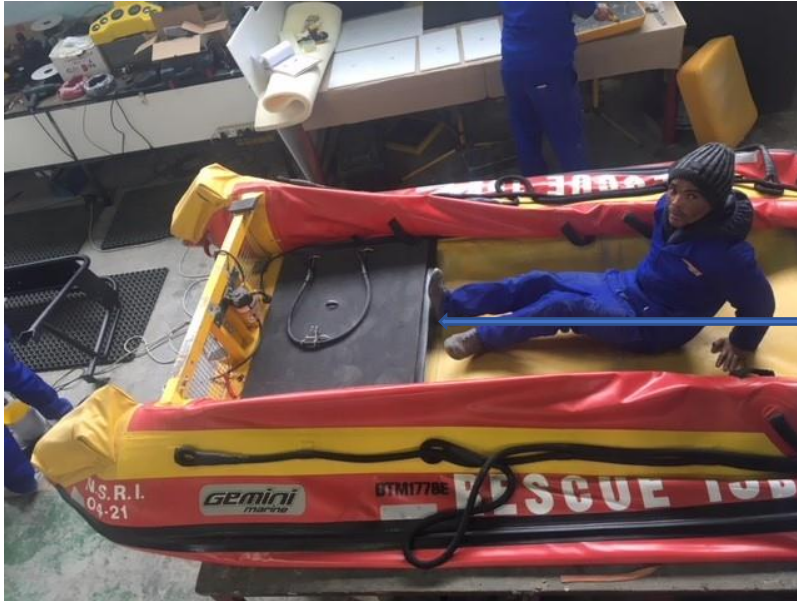
Aft floorboard (fifth floorboard) fitted snugly at transom and underneath the retaining rubbers.
